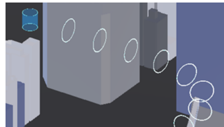
Fig. 4. Example of a predefined flight route, where sequential rings indicate the path and direction of movement.
