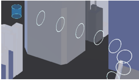
Fig. 3. Example of a predefined flight route, where sequential rings indicate the path and direction of movement.
